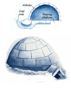
**Step 5.** Hot air from your body and stove rises and is trapped inside the dome. Cold air falls into the sink and flows away to the outside. It is essential to cut ventilation holes in the walls with an ice axe.
