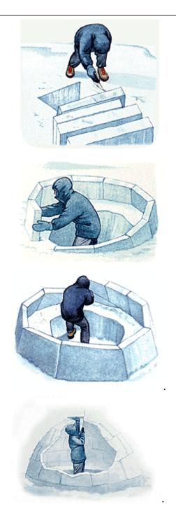
**Step 1.** Cut blocks from dry, hard, hard snow, using a snow saw or large knife. Each block should be about 3 ft. (1m) long, 15 in. (40cm) high, and 8 in. (20cm) deep.
