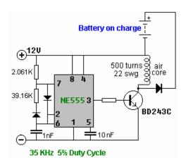
Here, the coil is wound with 500 turns of 0.7 mm enamelled copper wire and the actual construction is compact:
