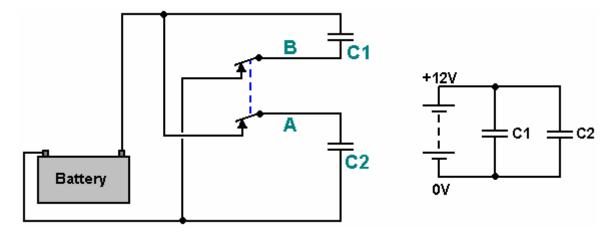
As you can see, the "normally closed" relay contacts have each of the capacitors connected directly across the battery supply rails. This gives the circuit shown above on the right. When the relay is powered up, the situation changes very suddenly to give this arrangement:
