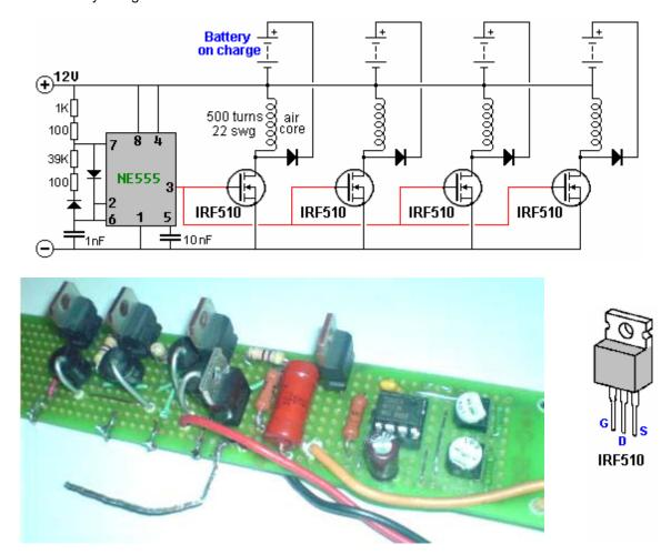
While these coils are air-core to allow high frequency operation, coils are generally much more efficient with some form of magnetic core, such as iron-dust or ferrite. While it is not likely to be able to operate at frequencies as high as 35 KHz, a very good material for coil cores is the metal of masonry anchors or "sleeve anchors":
