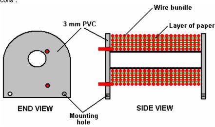
The coils are wound with the end plates attached and drilled ready to screw to their 1/4 inch (6 mm) PVC bases, which are the bolted to the 3/4 inch (18 mm) MDF supporting structure. To help the winding to remain completely even, a piece of paper is placed over each layer of the winding:
