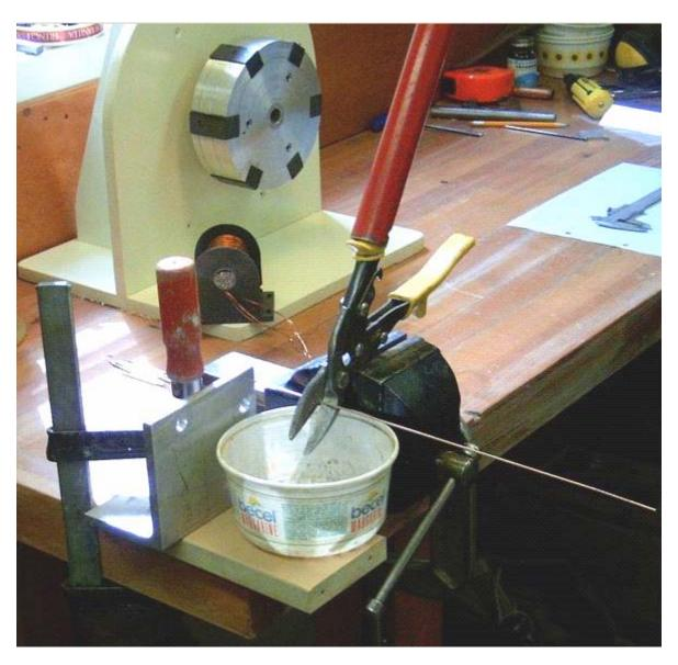
The distance between the shears and the metal angle clamped to the workbench makes each cut length of wire exactly the required size while the plastic container collects the cut pieces ready for coating with clear shellac or clear polyurethane varnish before use in the coil cores.
