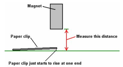
Having graded the magnets in order of strength, Ron then took the best twelve and paired them off, placing the weakest and strongest together, the second weakest and the second strongest, and so on. This produced six pairs which have fairly closely matching magnetic strengths. The pairs of magnets were then glued in place in the rotor using super glue:
