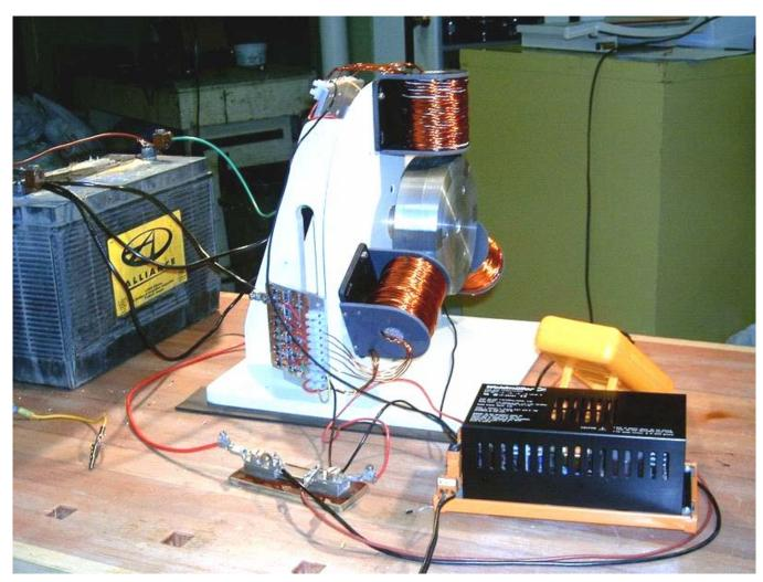
This is not a toy. It draws significant current and produces substantial charging rates. This is how Ron chose to build his device. The rotor is constructed from aluminium discs which were to hand but he would have chosen aluminium for the rotor if starting from scratch as his experience indicates that it is a very suitable material for the rotor. The rotor has six magnets inserted in it. These are evenly spaced 60 degrees apart with the North poles all facing outwards.
