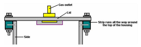
A gasket, perhaps of flexible PVC, placed between the sides and the lid would assist in making a good seal when the lid is bolted down. The gas outlet pipe is located in the centre of the lid which is a position which is not affected if the unit is tilted when the vehicle is on a steep hill.
