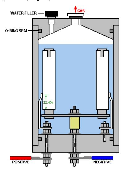
This cross-sectional view may be slightly misleading as it suggests that each of the nine outer pipes has its own separate bracket and this is probably not the case as they are connected together electrically through the steel ring-shaped disc and should vibrate as a single unit. It is tempting to use separate brackets as that would allow the assembly to be taken apart quite easily, but the electrical contacts of such a system would be much inferior and so it is not to be recommended.
