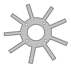
This piece has four holes drilled in it to match the stud positions of the plastic base piece. The number of studs is not specified and while I have shown four, the plate resonance might be helped if there were just three. The size is arranged so that when the arms are bent upwards at right-angles, they fit exactly against the inner face of the acrylic tube.
