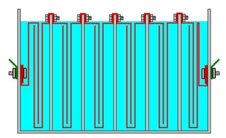
While this six-cell design may look a little complicated to a quick glance, it is really a very simple construction. Each of the plates used in the central cells is just this shape:
