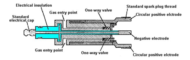
This cross-section shows only two of the three entry points through the injector as they are spaced 120 degrees apart, and so the third one is not seen. Each of these has its own one-way valve so that when the pressure inside the cylinder is raised during the compression and power strokes, no flow back along the feeder tubes occurs. The
