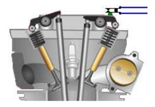
An alternative is to attach a strong permanent magnet to the rocker arm, using epoxy resin, and then position a solid state "Hall-effect" sensor so that it triggers the delay before the spark is generated.
