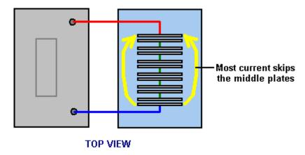
This is a disaster for us as now we will not get your six times the gas production or our massively reduced heating. Thankfully, there is a very simple fix for this problem, and that is to divide the box up into six watertight compartments using thin partitions like this:
