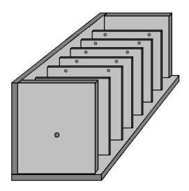
Here, the partitions are fixed in place one at a time, and finally, the second side is attached and will mate exactly as the partitions and ends are all exactly the same width. A simple construction for the lid is to glue and screw a strip all the way around the top of the unit and have the lid overlap the sides as shown here:
