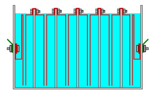
Any of these designs can be 6-cell or 7-cell and the plates can be constructed without outside help. You will notice that the electrical connections at each end of the booster are submerged to make sure that a loose connection can't cause a spark and ignite the hydroxy gas in the top of the housing. There should be a gasket washer on the inside to prevent any leakage of the electrolyte past the clamping bolt.
