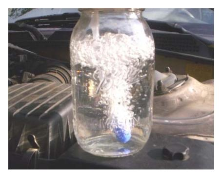
The unit is attached to the air intake of the vehicle, between the air filter and the engine. A small diameter plastic pipe is lead from there to a glass or plastic container holding water. In the above picture Roger is using a glass Mason jar with a screw-on metal lid which has a seal. Sometimes called a preserving jar, these jars are very convenient.
