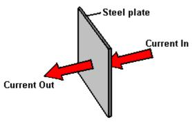
The fact that we have folds and bends in our plates has no significant effect on the current flow. Resistance to current flow through the metal electrode plates is something which can't be overcome easily and economically, and so has to be accepted as an overhead. Generally speaking, the heating from this source is low and not a matter of major concern, but we provide a large amount of plate area to reduce this component of power loss as much as is practical.
