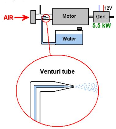
It is just a pipe which tapers to a point and which has a very small nozzle. As the engine draws in the air/hydroxy mix on it's intake stroke, the mixture rushes past the nozzle of the Venturi tube. This creates an area of lower pressure outside the nozzle and causes water to exit through the nozzle in a spray of very fine droplets. Some perfume spray bottles use this method as it is both cheap and effective.
