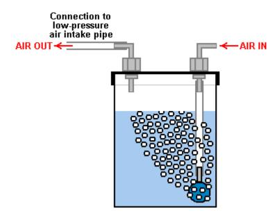
The container has a plastic elbow connection in the lid through which the outside air is drawn into the container. The air flows down through a plastic tube to either an air-stone from a pet shop, or a loose bolt in the end of the plastic tube. The air-stone has many small holes in it and these break the incoming air up into many streams of small bubbles.
