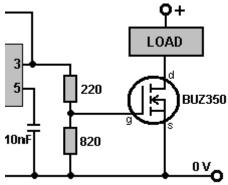
Here, the 555 chip output voltage is lowered by 220 / 820 or about 27%. When the voltage rises, it causes the BUZ350 transistor to switch on, short-circuiting between its Drain and Source connections and applying the whole of the 12-volt supply voltage across the load, which in our application, is the electrolyser cell:
