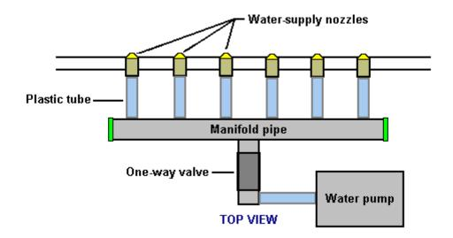
A point which might not be immediately obvious is that because the gas pressure inside the booster is probably about 5 pounds per square inch ("psi"), once the water pump stops pumping, it is possible for the gas pressure to push out the remaining water in the inlet pipes and escape through the body of the pump. To prevent this, an ordinary one-way valve is put in the water supply pipe to prevent flow back towards the pump.
