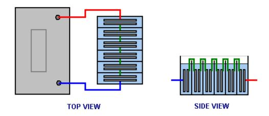
This gives us back our high efficiency by blocking the current flow past the plates and forcing the current to flow through the plates, producing gas between every pair of plates.
