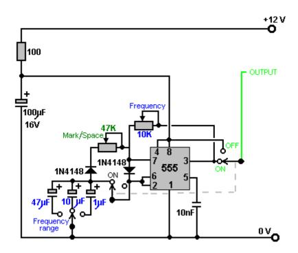
which just has one additional switch to allow the output to be stopped and the 12-volt supply line to be fed instead. The reason for this is that this part of the circuit is used to switch On and Off an identical circuit. This is called "gating" and is explained in Chapter 12 which is an electronics tutorial.
