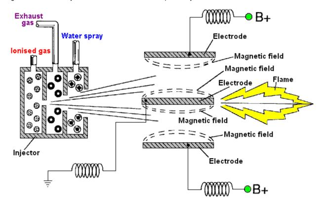
One component is described as ionised gas and ambient air is mentioned. The second component is part of the exhaust gas which is hot water vapour fed through a limiting valve, although inert gases are also mentioned. The third injection component is a very fine spray of water droplets or "mist". This mixture is passed between high voltage electrodes and if the mix does not ignite spontaneously, then it is ignited with a spark.
