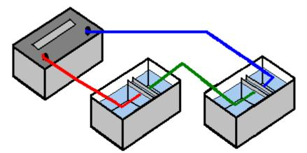
This arrangement uses our 1.24 volts twice while the twelve volts stays unchanged and so the electrical efficiency goes up to 20% and the heat loss drops to 80%. That is quite an improvement but even more important is the fact that twice as much hydroxy gas is now produced, so we have doubled the electrical efficiency **and** doubled the gas output, giving a result which is four times better than before.
