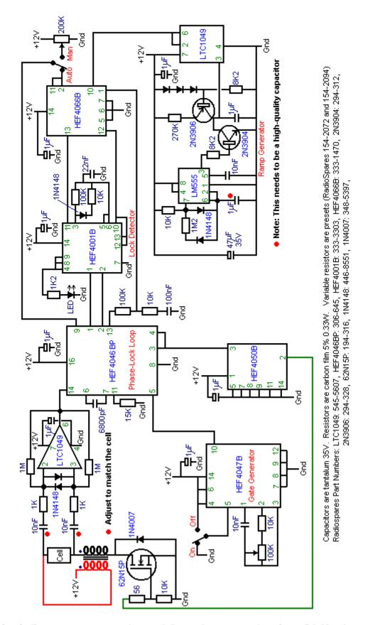
Note: This circuit diagram was corrected on 28th December 2009 and again on 5th March 2010 where the output pin of the HEF 4047B was swapped from pin 11 to pin 10 to use the alternative output signal.
