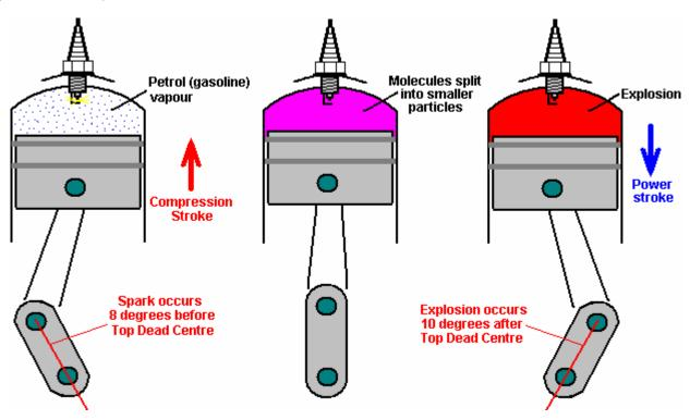
If you were to replace the petrol vapour with hydroxy gas, then there would be a major problem. This is because hydroxy gas has very small molecule sizes which do not need any kind of breaking down and which burn instantly with explosive force. The result would be an explosion which occurs far too soon and which opposes the movement of the rising piston as shown here:
