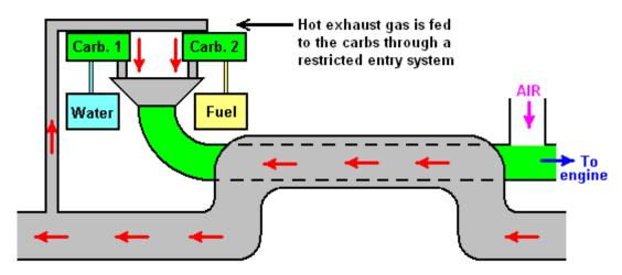
The use of carburettors is important since using a bubbler as suggested in the free plans on the internet, creates problems as the lighter fractions of the fuel get taken first which is exactly what we don't want to happen. The carburettors have the massive advantage that they feed all fractions of the fuel together and so the remaining fuel is always in the correct proportions.
