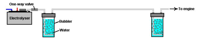
Where the first bubbler is close to the booster and the second one is placed close to the engine. Once in a while, the water from the first bubbler can be used to top up the water inside the booster so that any traces of hydroxide
