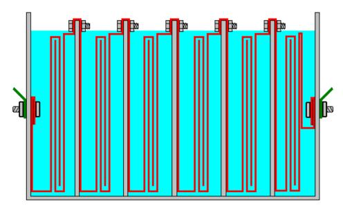
The electrolyte is a mix of water and an additive to allows more current to flow through the liquid. Most of the substances which people think of to use to make an electrolyte are most unsuitable, producing dangerous gasses, damaging the surfaces of the plates and giving uneven electrolysis and currents which are difficult to control. These include salt, battery acid and baking soda and I strongly recommend that you do not use any of these.
