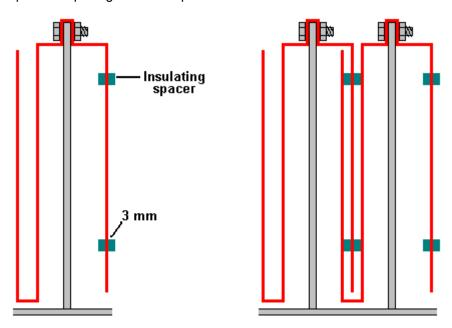
If the current is low enough, an even more simple shape which has just a single pair of active plate surfaces per cell, can be used as shown here:
