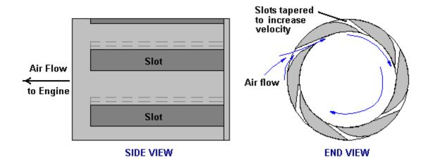
The air enters through each of six tapered slots cut parallel to the axis of the pipe. These give the air an initial spin inside the pipe and the pulsating intake of the engine, combined with the oval shape of the PVC exit T-piece, accelerates the air into a serious vortex which improves the intake to the engine, raising it's efficiency and giving more engine power.
